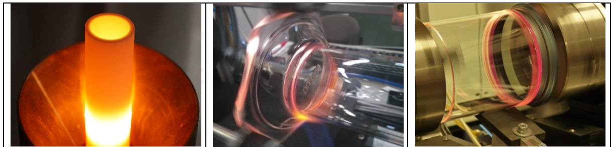
Fig. 4 Laser soldering \text{Al}_2\text{O}_3 ( \varnothing 20 mm), processing of measurement cylinder (500 ml) and glass-metal-bond ( \varnothing 120 mm)
