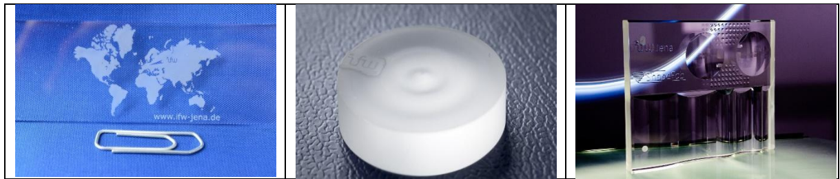
Fig. 5 Marking, ablating ( \varnothing 20\text{ mm} ) and laser polishing ( 180\text{ mm} \times 150\text{ mm} )
