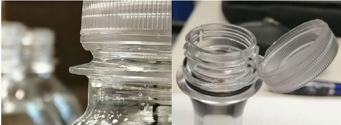
Fig. 3 Laser-sealed PET cap, shown on the right in the attached version components. To ensure that the melt volume is sufficient for a joint, the area around the weld seam is preheated with a gas burner or with a second laser beam, which increases the thermal conductivity.
