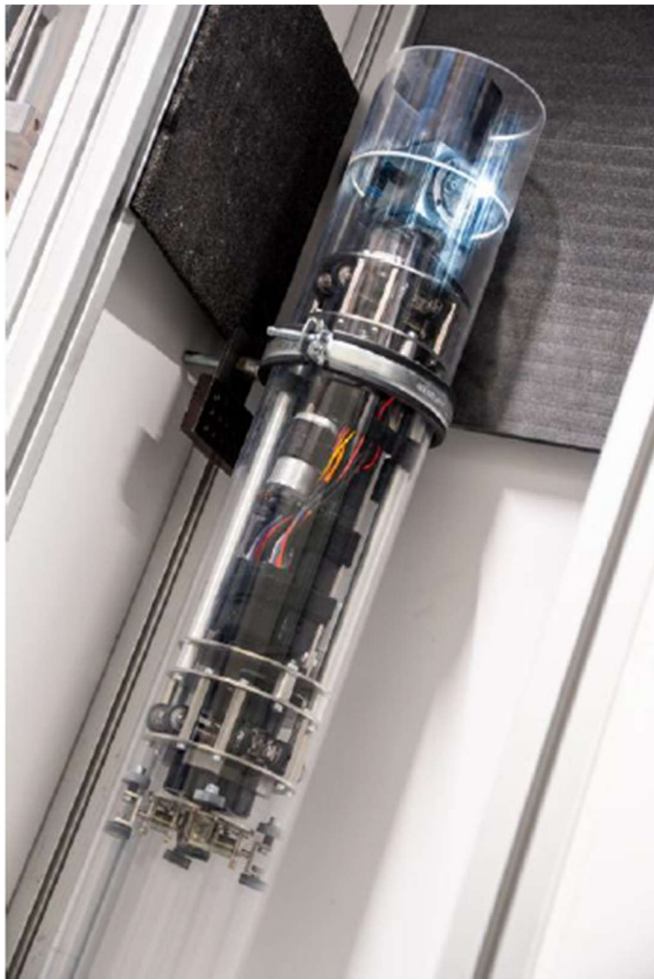
Fig. 2 Tube robot in laboratory testing: Laser cutting on a vertical quartz glass tube ( \varnothing = 100 mm, s = 3 mm)
