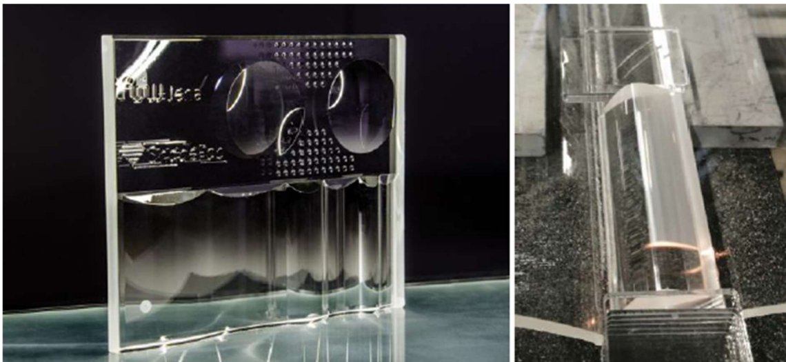
Fig. 1 Laser polishing of glass; on the left, a borosilicate glass plate (180 mm x 150 mm); on the right, a quartz cylindrical lens (100 mm x 25 mm)
