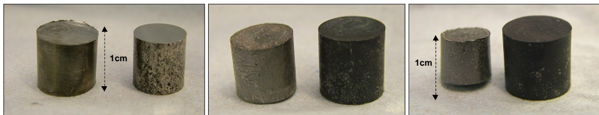
Fig. 8 Oxidation of molybdenum (left) versus CG iridium (Right)
