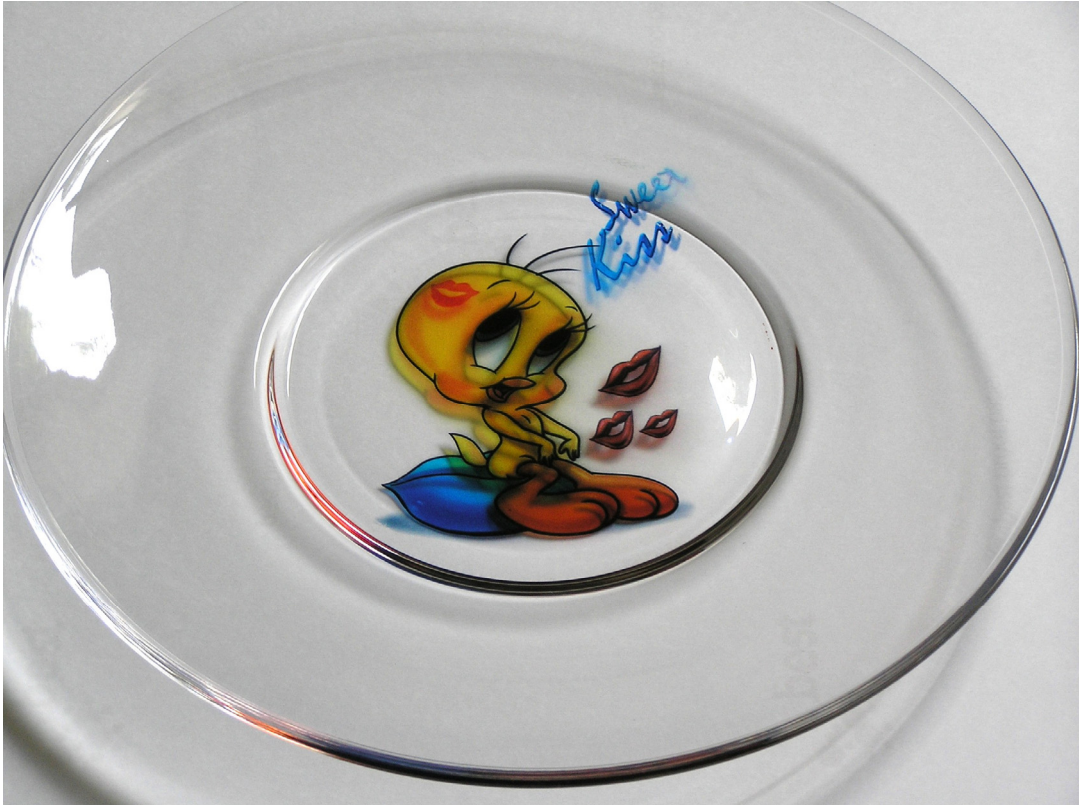
Fig. 19: Inkjet print on a glass plate with Ormojet hybrid ink, printed with a Technoplot printer
